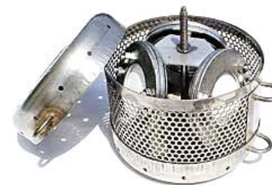
POCIS (Polar organic Chemical integrative sampler), log kow 1-4 (Wang et al., 2020)
